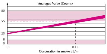
Typical Response Characteristic - XP95 Optical Smoke Detector
